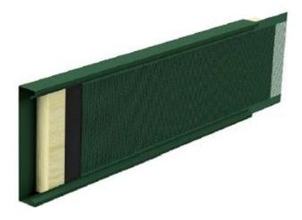
The sound insulation panels consist of two metal plates assembled with a joint without screws. The steel sheet with special corrosion protection is electrostatically painted and resistant to atmospheric conditions. The sound function barrier is provided by the inner core with a special sound absorbing material 70mm thick and  $70 \text{kg/m}^3$ . The rear panel provides sound reduction while the front is perforated 36% and helps absorb sound.
